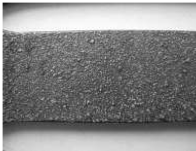
Fig. 3. The appearance of the sample surface strengthened by alloy T15K6
